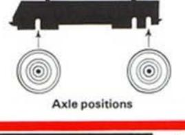
When assembling the non-powered bogie ensure that the insulated wheels (shaded centres) are on the correct side.
